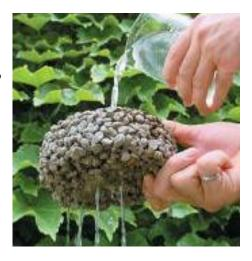
Pervious pavement reduces the ability of pollutants to build up. Pervious pavement uses the same materials as conventional concrete, but the fine aggregate material found in conventional concrete
